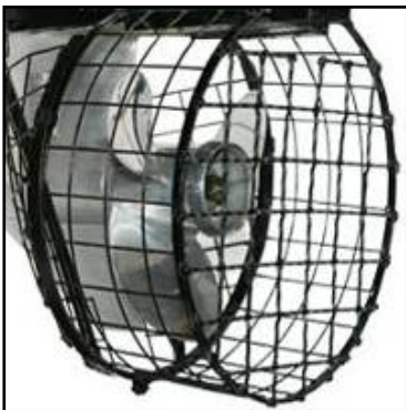
Examples of allowable propeller guards
